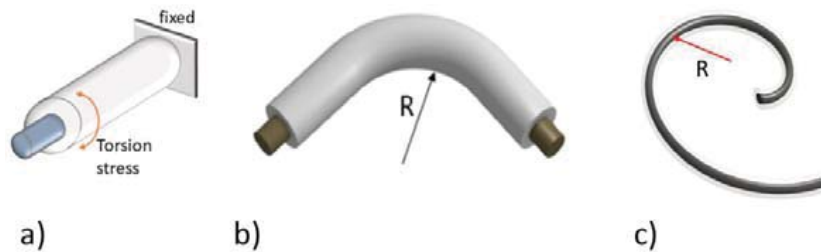
Fig. 1. Torsion (a), bending (b) and spiral (c) mechanical stresses applied to the studied microwires.
